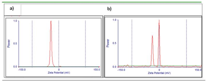
Fig 3. Zeta potential of freshly prepared green tea-extract synthesized AgNPs (a) and black tea-extract synthesized AgNPs (b) with  $\zeta$  values -30 mV and -19mV, respectively.
